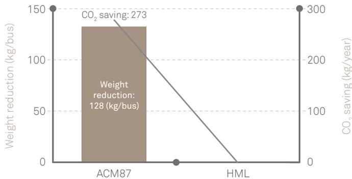
a) comparing against a HML core (2500 kg/m<sup>3</sup>), in a configuration 6/3/6 an 500kg/m<sup>3</sup> plywood
